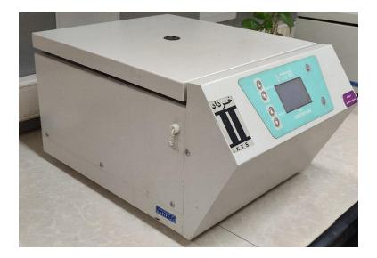
FacilityCentriFugeManufacturerKTSSample Holders2ml MicrotubesRotational Speed8000-15000RPM
